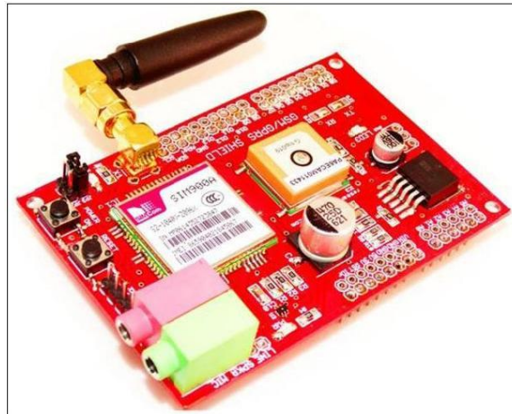
Fig. 6.The SIM900A GSM /GPRS with GPS receiver module.
